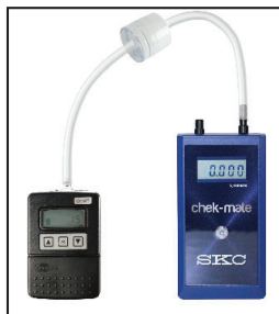
Flow rate verification train with filter cassette
