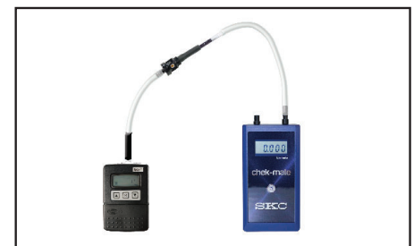
Flow rate verification train with All-in-One
